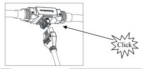
NOTE: AC connector interface as follows, from left to right PE, N, L3, L2, L1.
