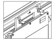
Step 4. Connect the APsystems Microinverter cables to the AC bus cable.
