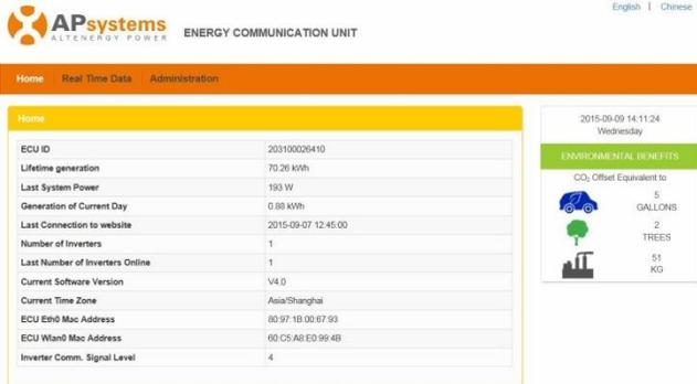
The screenshot displays the APsystems Energy Communication Unit (ECU) web interface. At the top, there is a navigation bar with 'Home', 'Real Time Data', and 'Administration'. The main content area is divided into two sections. The left section, titled 'Home', contains a table of system parameters. The right section, titled 'ENVIRONMENTAL BENEFITS', shows the CO<sub>2</sub> Offset Equivalent to 5 GALLONS, 2 TREES, and 53 KG, accompanied by icons of a car, a tree, and a factory.
