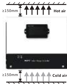
Fig. 2.1 Installation and Heat Dissipation
